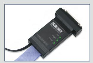
The Raven is a BDM/JTAG interface used in the design, debug, and programming of microprocessor and microcontroller based embedded systems. One side of the Raven interfaces to the parallel port of a host PC and the other side connects to an OCD (On-Chip Debug) port on the target system. As with all Macraigor interface devices, the Raven can simultaneously debug up to 255 devices on a single scan chain.
